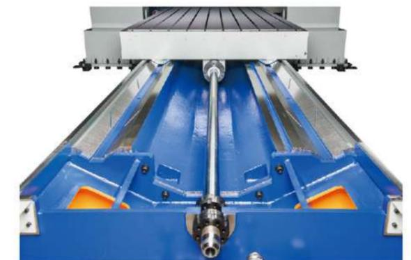
**X-axis Driven by Hydraulic Cylinder**
