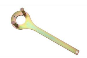
\* Brake loose the crank shaft pulley/harmonic balancer bolt. Designed to properly secure the pulley from rolating during R & R of crank bolt. The 50mm hex head armature slips past the lightest of spaces and slides right into the center slot on the pulley. Then slide the long bar onto the receiving end of the armature and lock it into position with the securing bolt
