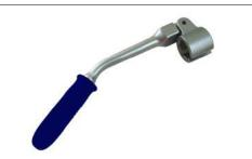
Angled Socket 22mm hex Application: VW-Audi, BMW, Mercedes, Ford, Opel/Vauxhall, Peugeot, Citroën, Renault, Seat, Skoda, Japanese cars, etc. Angle bent at 30o 12\*12-point: 22mm Length: 250mm Weight: 450g
