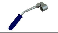
Angled Socket 22mm hex Application: VW-Audi, BMW, Mercedes, Ford, Opel/Vauxhall, Peugeot, Citroën, Renault, Seat, Skoda, Japanese cars, etc. Angle bent at 30o 12\*12-point: 22mm Length: 250mm Weight: 450g
