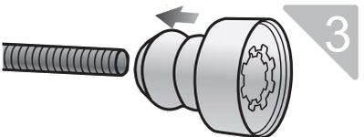
Use the gear-key and 21mm socket wrench to tight up the lock body.
